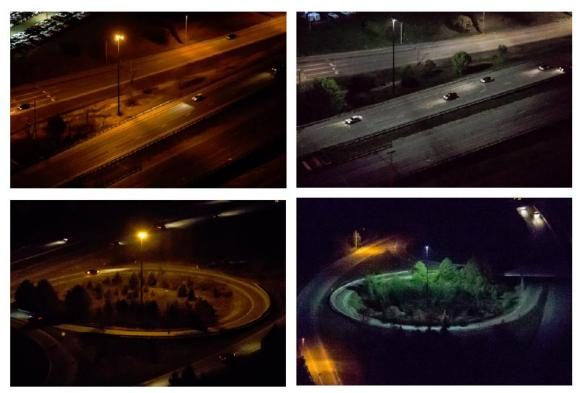
The above photo shows areas of I-295 in Portland with different levels of Kelvin lighting. The photos on the left are high-pressure sodium lighting of 2100 Kelvin. The picture on the right represents the full cut off 4000 Kelvin lighting. As shown above, the 4000 Kelvin lighting provides more contrast to vehicles and pedestrians.
