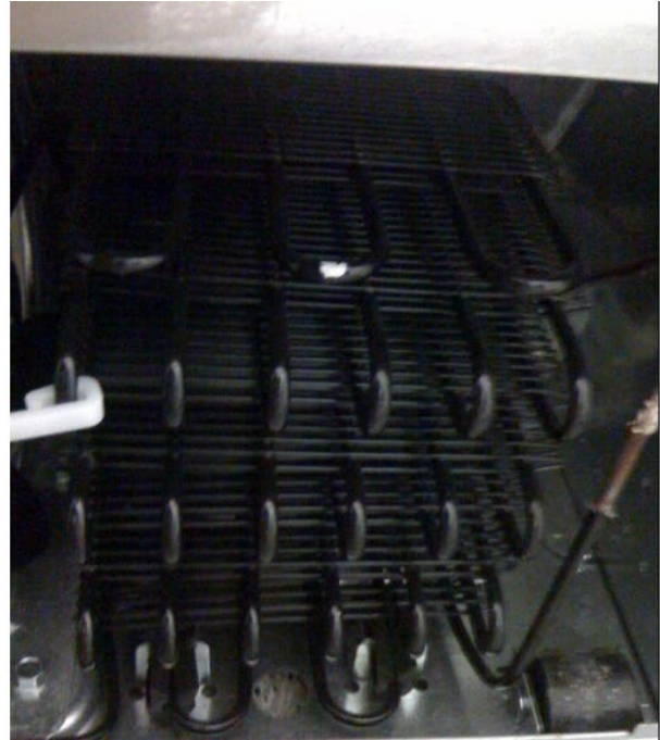
Standard back of the cabinet condenser Energy Star condenser packed under cabinet
