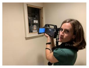
Melissa Ostroff used an optical gas imaging camera to see a methane leak from the gas meter in her basement.
