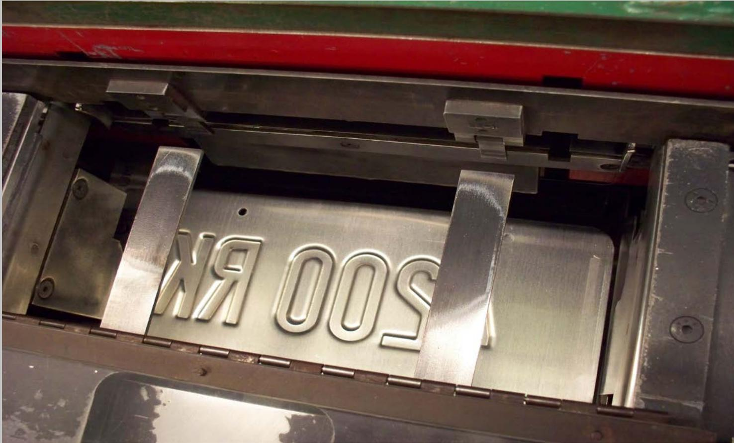
The embossed plate is face down and has received the impression of the die set characters and a rim.
