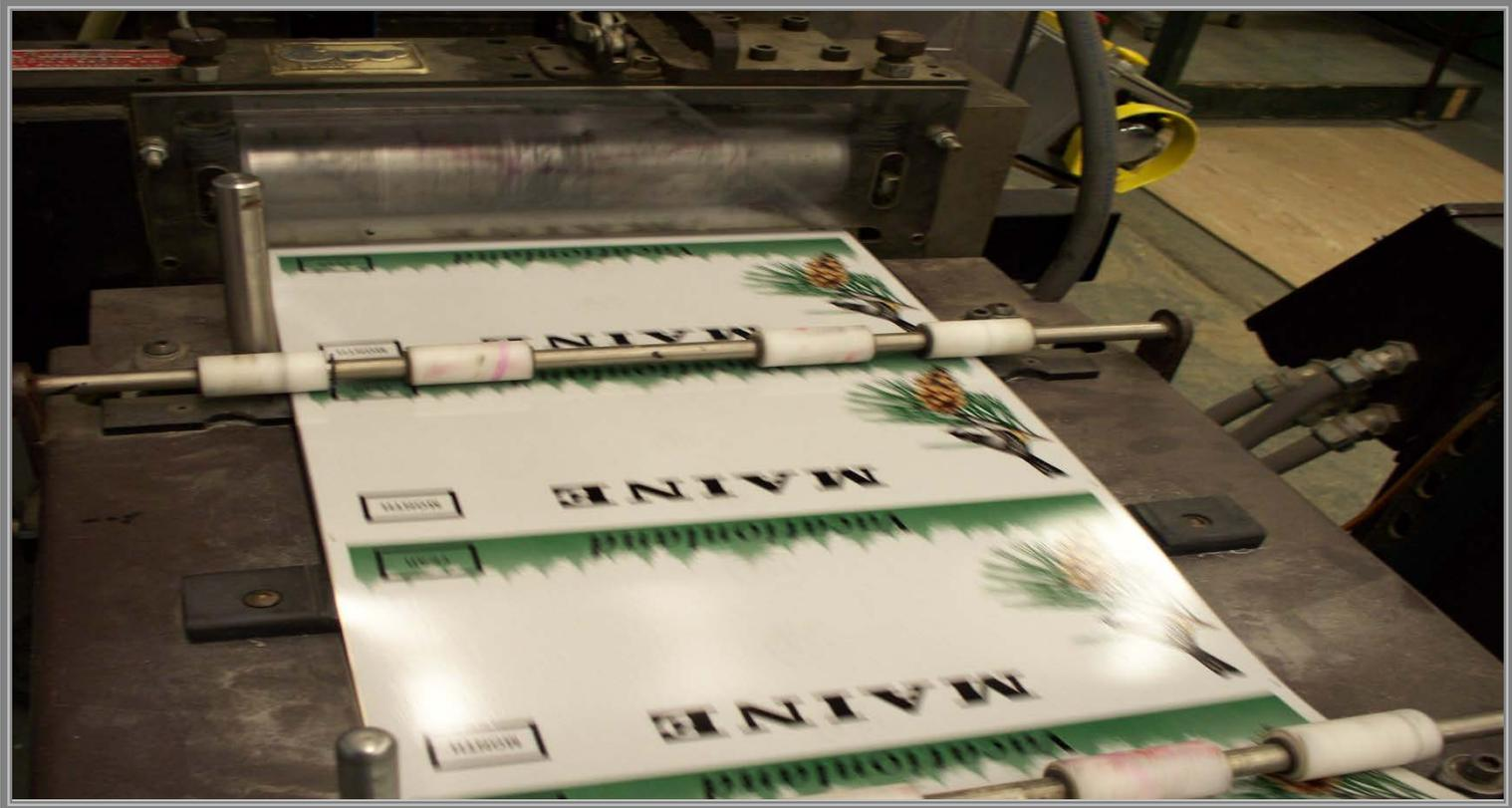
At this point, no rims, no letters or numbers are embossed, only the Scotchlite has been applied and the corners trimmed, and the holes punched.
