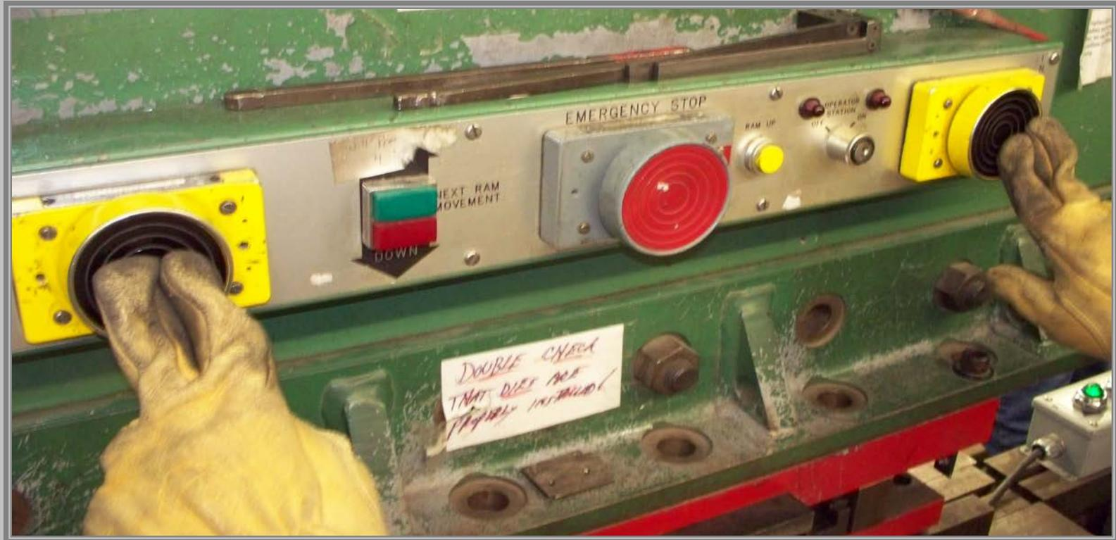
This process is repeated for each blank in conjunction with the operator changing the rotation of the die characters to maintain a numeric series of license plates.
