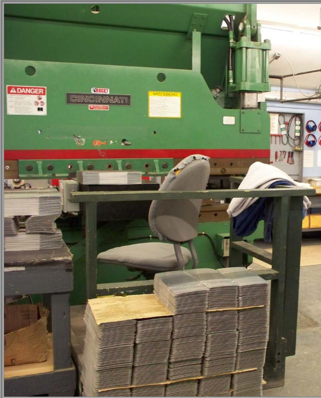
The Embossing Press creates the rims, numbers, and letters onto the blank plates. It takes three people to operate the Embossing Press. One to feed the machine, one to operate the machine and dies, and one to catch the plates from the conveyor belt and stack them.
