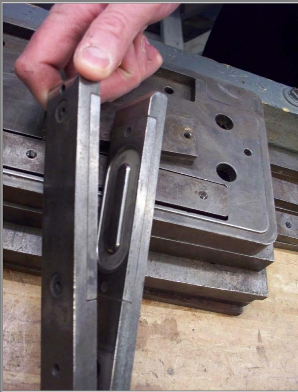
This die is the number "0". The embossing die resembles a giant clothes pin without the spring. It has a limited opening and is inserted in its place on the Embossing Press by the operator. When inserted into the Embossing Press, the blank sets inside this die, allowing the force of the machine to emboss the image into the blank.
