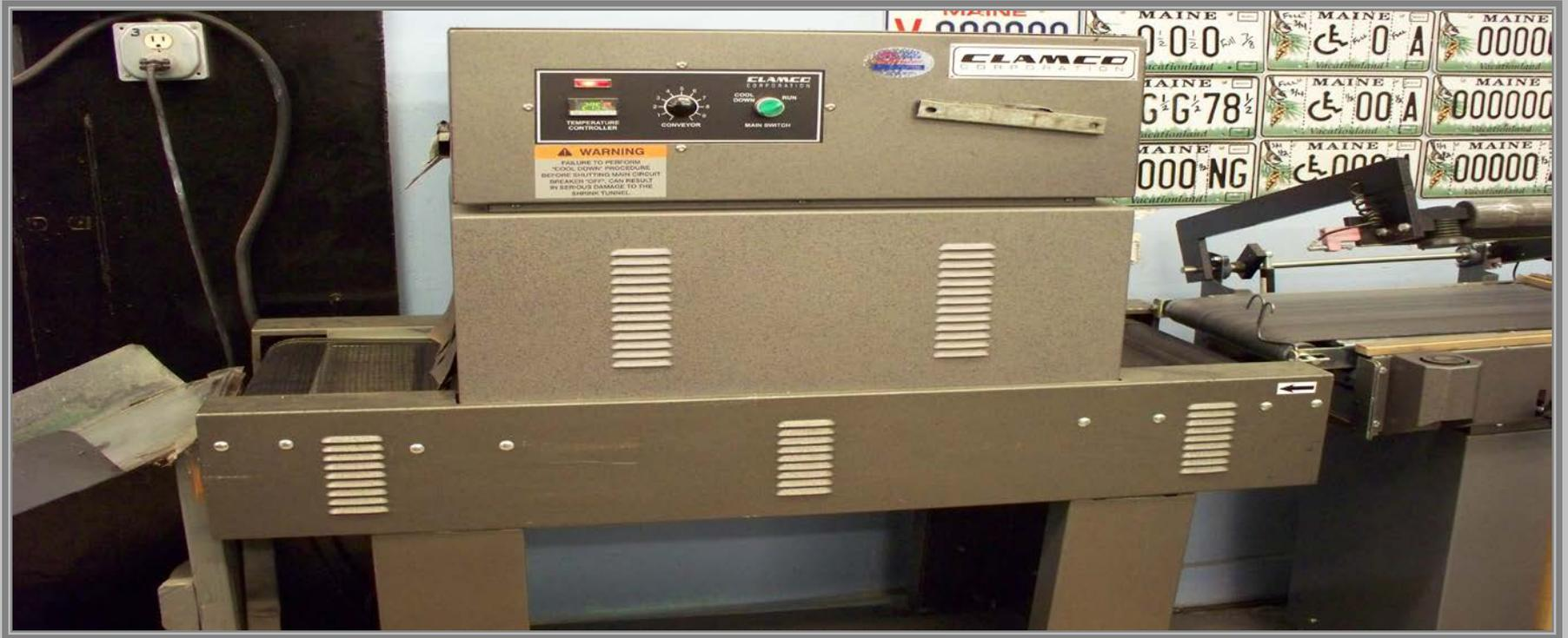
Pairs of plates must be brought to the Sealing Machine before receiving strapping. Each pair is placed on a tray and cellophane is wrapped around them. The pair proceed into the Sealer that shrink wraps the plastic to the plates as the sealed wrapped pair exits from a conveyor belt, down a shoot, and ready for bundling.
