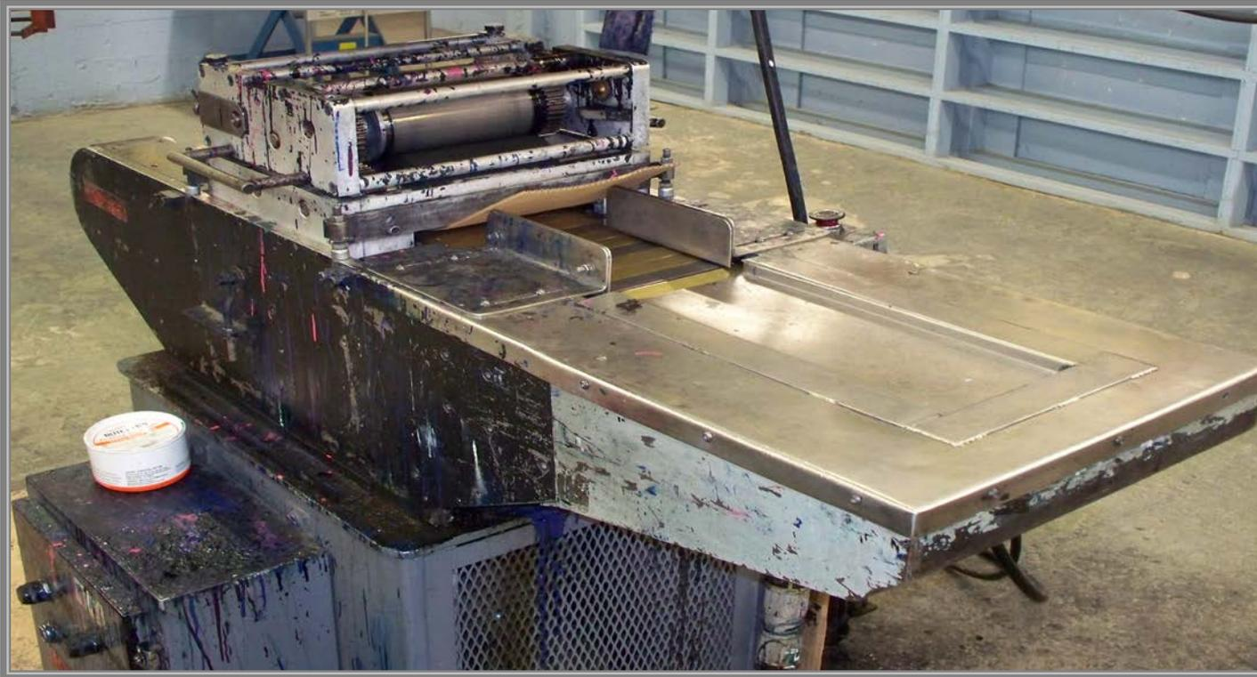
The Inking Machine was installed during this decade and uses oil-based ink. Each plate is inserted manually. The automated rollers pass over the raised characters to add color to the embossed Scotchlite.
