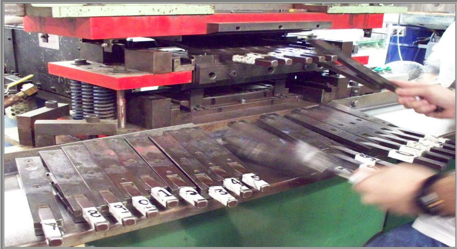
The blank has been set into position and ready for embossing. The operator inserts one hinged die for each character placeholder necessary to create a license plate. (Spaces included). He swaps dies between those waiting on the shelf to those inserted above the shelf in the Embossing Press.
