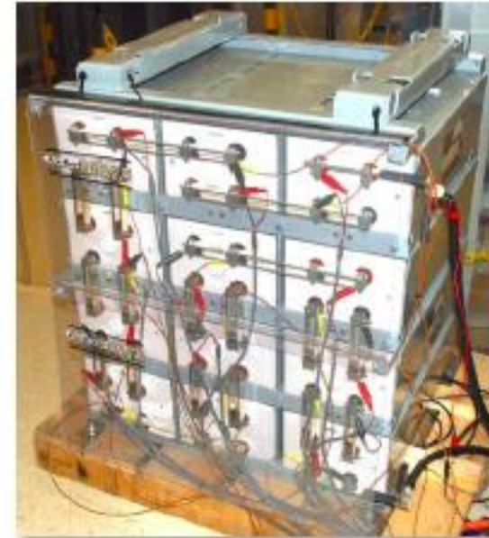
EastPenn Ultra Battery: 90% capacity at 20,000 cycles
