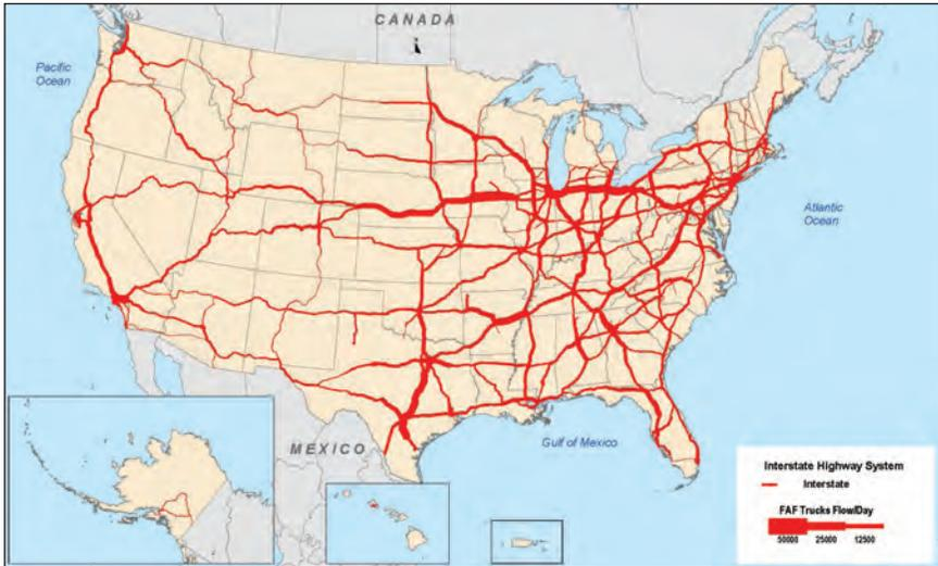
FIGURE 2-4 Average daily long-haul truck traffic on the Interstate Highway System, 2015.
