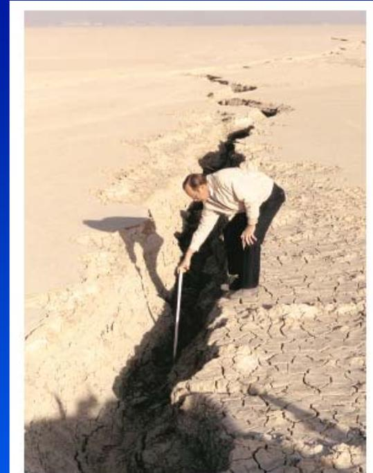
This earth fissure formed on Rogers Lake at Edwards Air Force Base, California, in January 1991, and forced the closure of one of the space shuttle's alternative runways. The fissure has been attributed to land subsidence related to ground-water pumping in the Antelope Valley area (Galloway and others, 2003).
